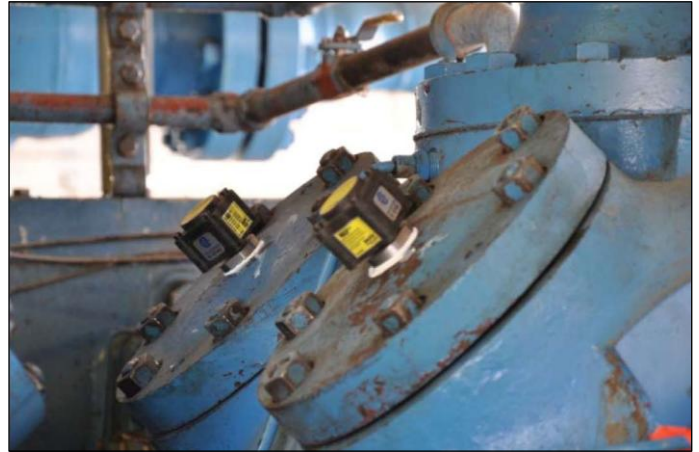
WASP™ sensors on a White Superior MW64 Gas Compressor
