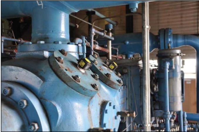
WASP™ sensors on a White Superior MW64 Gas Compressor
