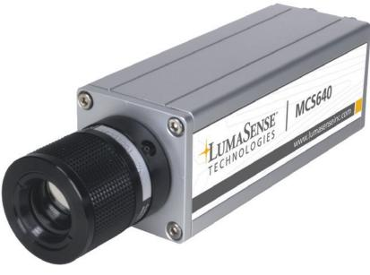
The MIKRON MCS640 from LumaSense Technologies, Inc., is a short wavelength infrared (SWIR) thermal imager with internal digital signal processing. This imager is designed to accurately measure temperatures between 600 and 3000°C, with minimal interference from temperature reflections on the object. This makes it suitable for applications such as measurements on metallic surfaces, graphite and ceramics, etc.
