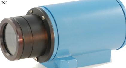
The MIKRON MCS640-HD from LumaSense Technologies, Inc., is a short wavelength infrared (SWIR) thermal imager with internal digital signal processing. This imager is designed to accurately measure temperatures between 600 and 3000 °C, with minimal interference from temperature reflections on the object. This makes it suitable for applications such as measurements on metallic surfaces, graphite and ceramics, etc.
