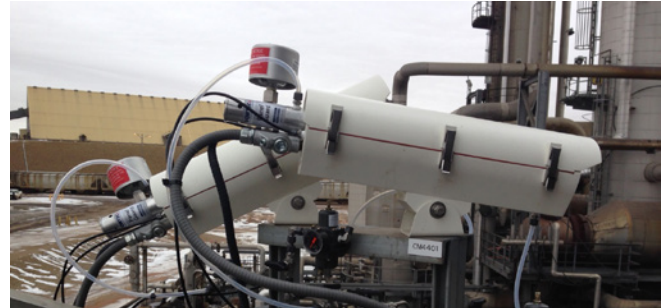
The ThermalSpec in its protective enclosure. Power, communication, and air connections are contained in a single hose.
