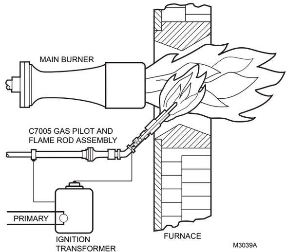
**Fig. 5. Typical mounting of gas pilot and flame rod assembly on inspirating (Venturi type) gas burner.**
