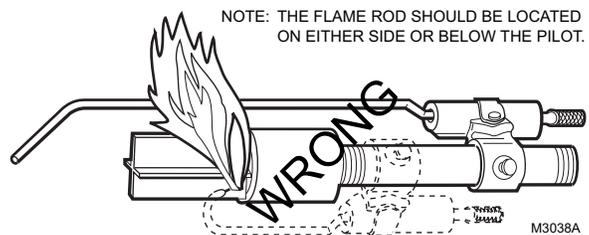
Fig. 2. Improper position of flame rod assembly in in. (mm).
