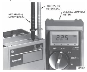
Fig. 8. Measuring flame signal voltage of 7800 SERIES control.
