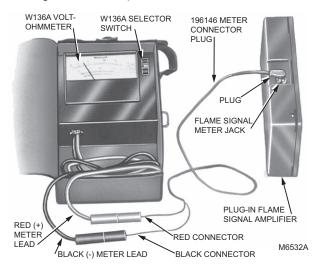
Fig. 7. Measuring microamp flame signal.
