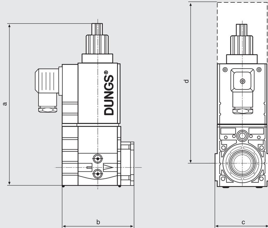
d = Space required for replacing solenoid
