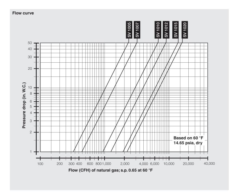
SV - Safety Shutoff Valve with Proof of Closure 1/2" NPT - 2" NPT
