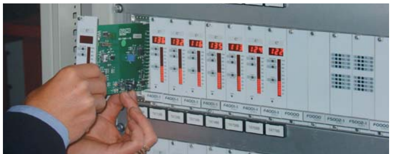
Hot swap of cards and power supplies, with no need for panel shutoff
