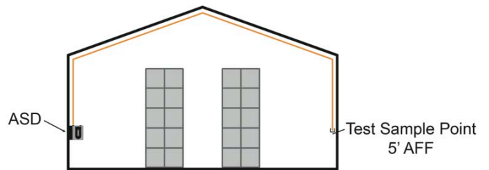
Figure 10. 3-Test sample point for warehouse installation
