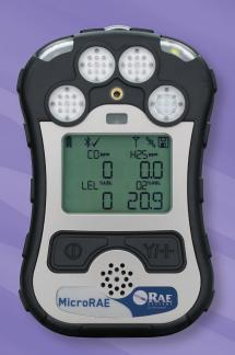
The MicroRAE four-gas portable detector brings enhanced userfriendliness and flexibility to wireless gas detection. This enables continuous, instant visibility of safety threats for faster, more informed decisions, to protect workers, facilities, and the environment, and to optimize operations.
