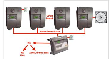
E³Point outputs directly to BACnet or other BAS. Alarms, strobes and horns are activated through BAS with link to DCV/HVAC controls. This system design supports new and retrofit installations for large buildings, and can couple with a controller to effectively integrate wired system components. A relay output is provided as an option for activating ventilation directly (e.g. when fan is located in close proximity to detector).
