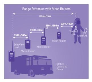
Mesh Router Enhances the Flexibility of the Wireless Solution
