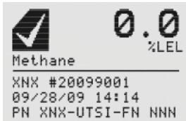
Figure 22. General Status Screen with Unit Information
