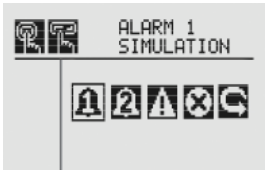
Figure 157. Alarm/Fault Simulation Menu
