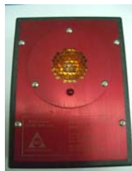
Figure 4-1 TL-1055 Hand Held Test Lamp (NEMA 1)
