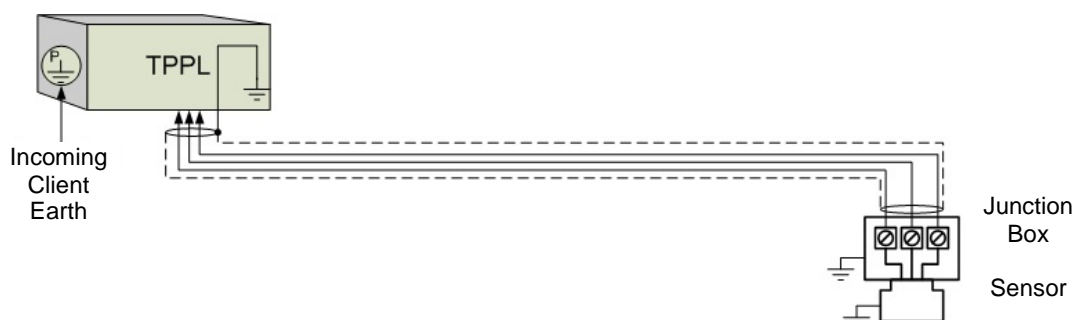
Figure 33. Grounding for Screened Cable, No Armour, with Metal Junction Box and Sensor
