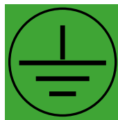
Figure 3 – Protective Earth (Ground) Point
