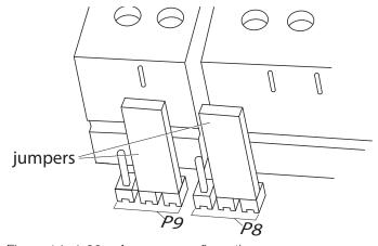
Figure 14. 4-20 mA source configuration
