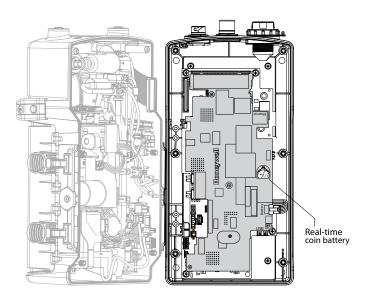
Figure 28. The real-time coin battery
