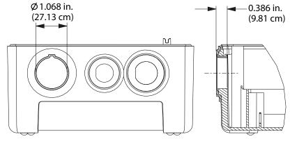
Figure 8. Ethernet opening dimensions
