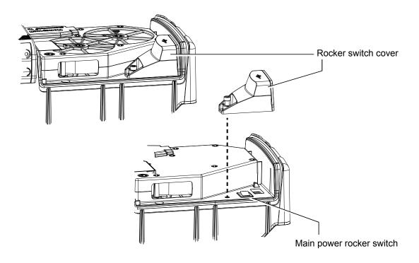
Figure 3. SPM Flex main power rocker switch
