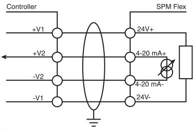
Figure 12. 4-20 mA isolated wiring diagram
