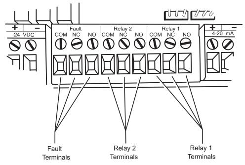
Figure 16. Relay configuration
