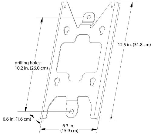
Figure 20. Standard mounting bracket
