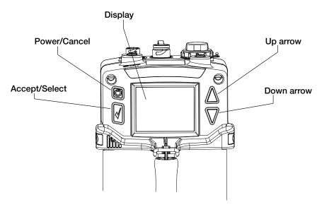
Figure 5. SPM Flex controls
