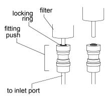
Figure 26. Removing a filter from a push fitting
