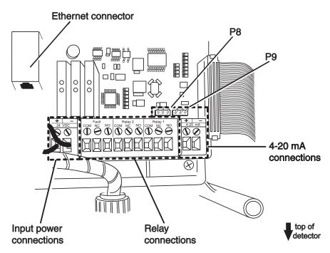
Figure 9. SPM Flex connections
