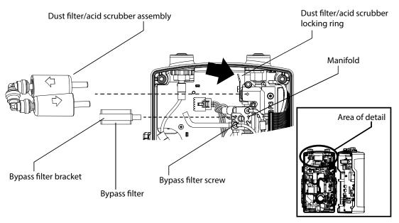
Figure 27. Removing the internal filters
