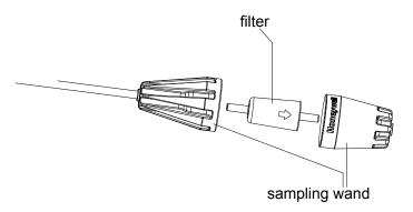
Figure 24. Wand with sampling filter
