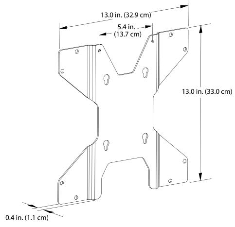
Figure 21. Backward-compatible mounting bracket
