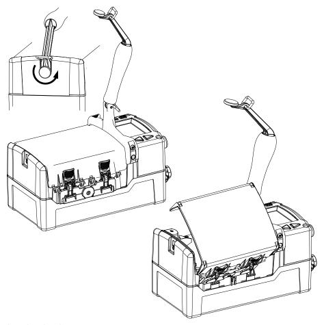
Figure 2. Opening the detector cover
