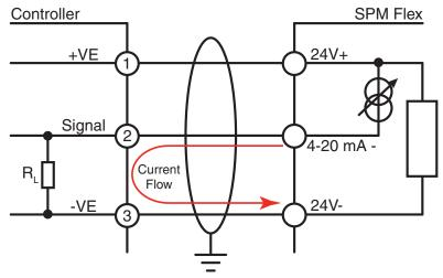
Figure 11. 4-20 mA source wiring diagram
