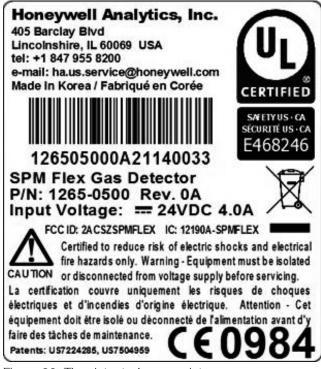
Figure 30. The detector's nameplate
