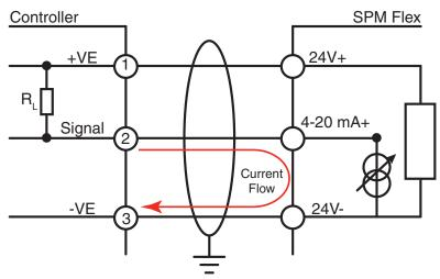
Figure 10. 4-20 mA sink wiring diagram
