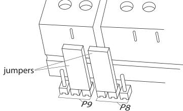
Figure 15. 4-20 mA isolated configuration (the default)
